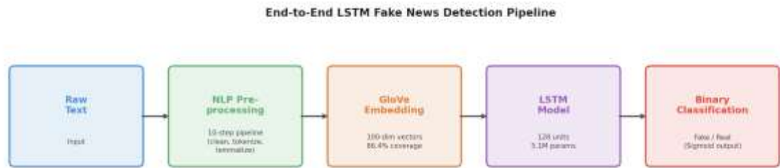
Figure 1. End-to-end system architecture for LSTM-based fake news detection
